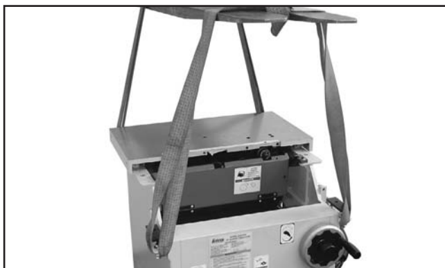
Figure 8. Lifting the table saw with a forklift and lifting straps (sliding table removed for clarity).
